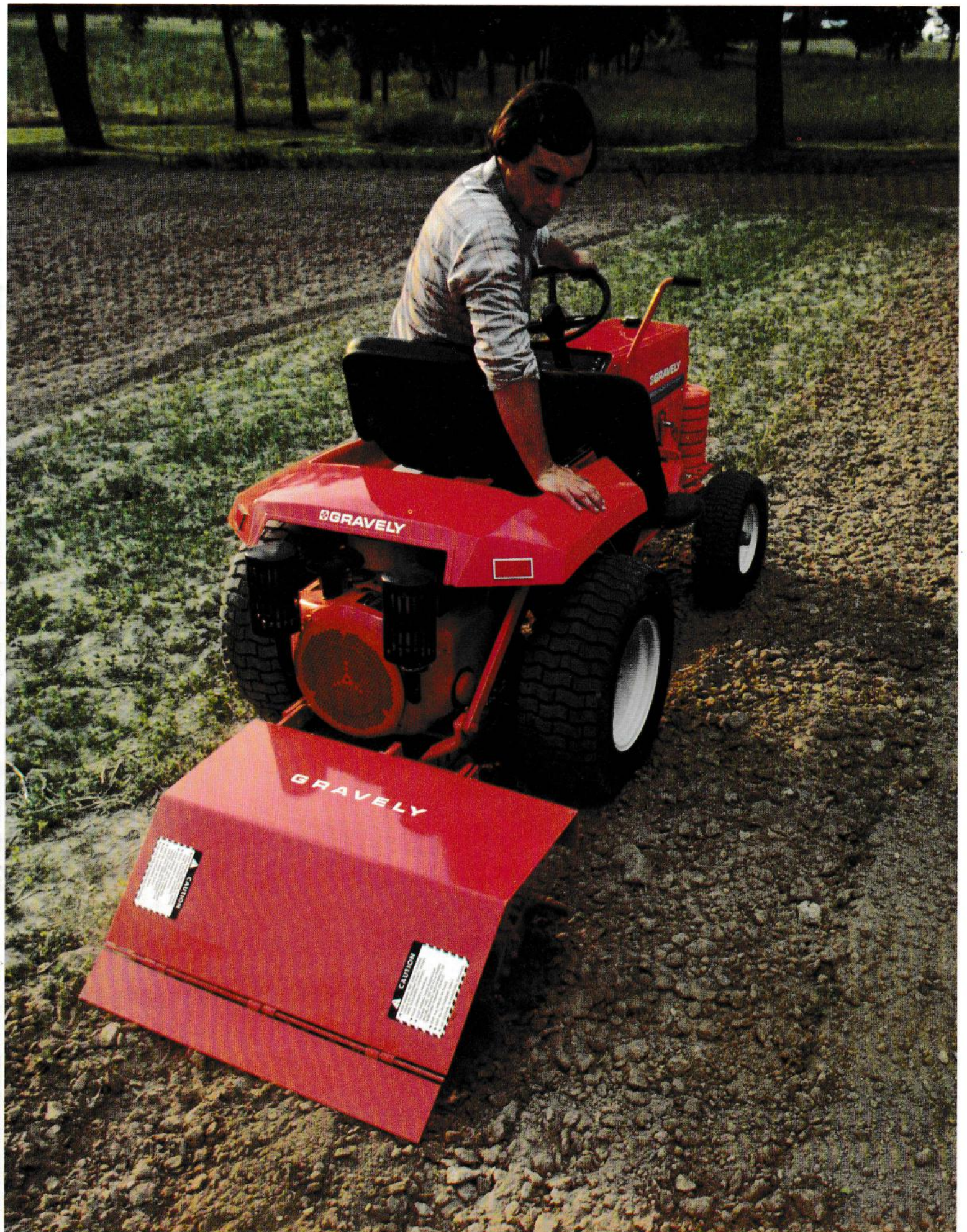
Gravely 8163-T, 16 hp Riding Tractor with all-gear and chain drive Rear Tiller, optional Rear PTO and Front Weight Rack with Weights.
