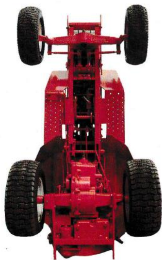
The all-steel, welded and reinforced box frame is built to absorb punishment from the tough jobs for years to come.
